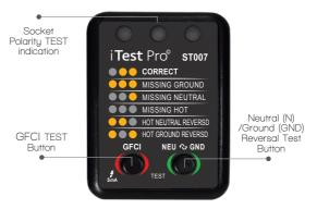
**Note:** The indicators will not illuminate if there is a wiring fault (missing Hot)
