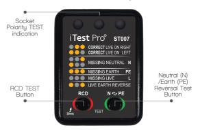
Note: The indicators will not illuminate if there is a wiring fault (missing L)
